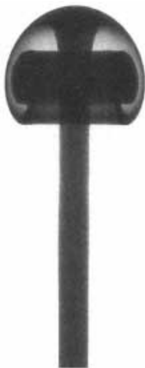
Fig. 7.17 Convection in viscous fluids at high Rayleigh number creates mushroom- shaped rising plumes. Such features are thought to exist in the Earth's mantle Where a plume breaks the crust, there is volcanism and an outflow of molten rock. (Photo: Ross Griffiths, Australian National University, Canberra.)
